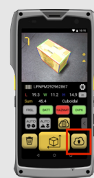
Save results to QBOID Cloud or another system (WMS, ERP, TMS, etc)
